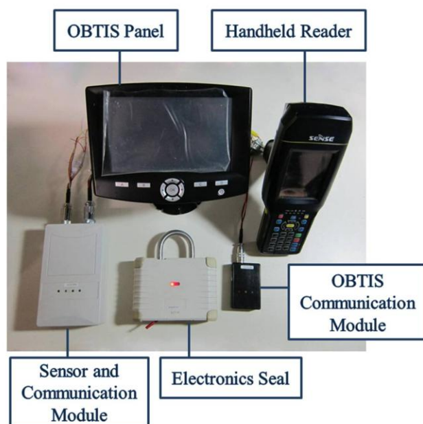
Photo 1: Main Components of an Intelligent eSecurity Device
