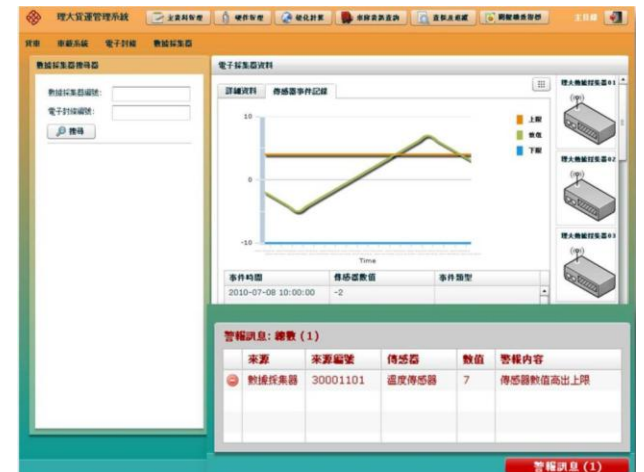
Photo 5: Fleet Management System automatically generates an alert message instantaneously when the temperature is out of range for immediate response action
