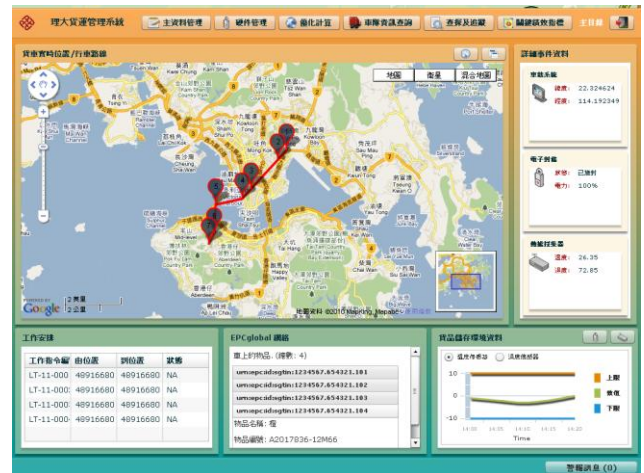
Photo 3: Fleet Management System - Real-time Conditions Tracking and Monitoring of Storage Environment
