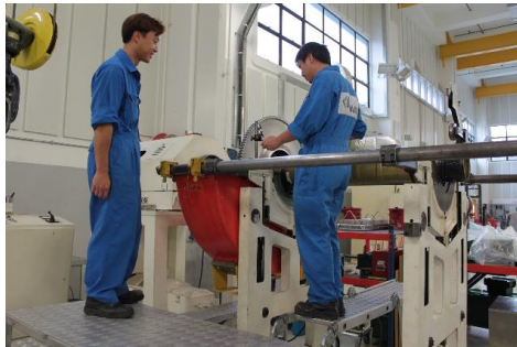
Photo 6: Preparing an Intermediate Pressure Turbine for balancing
