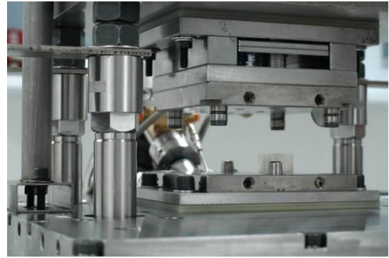
Photo 6: The first bottom-up high-precision plastic micro injection moulding machine.
