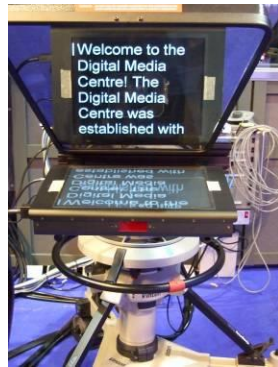
Photo 5: The newsreader is reading from this script monitor when he is looking at the camera.
