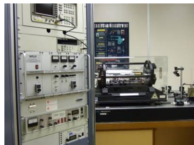
Photo 7: Iodine-stabilized laser for realization of metre
