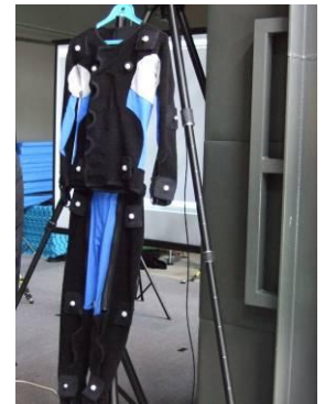
Photo 7: Motion capture suit with sensors allows 3D scanning and storage.
