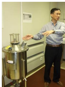
Photo 4: 50 l proving tank
