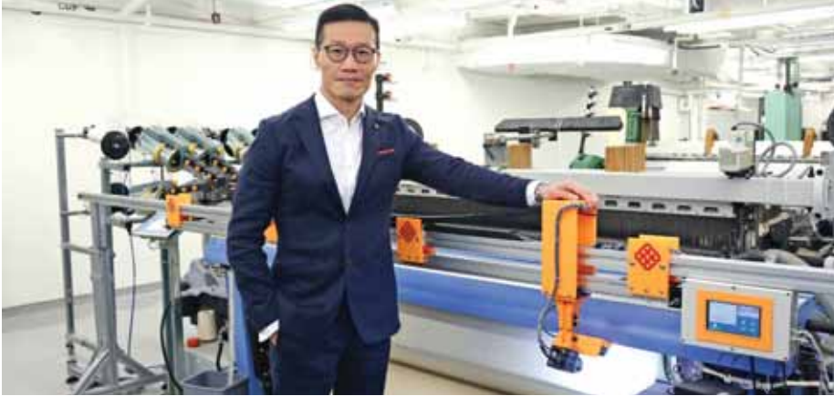
Prof. Calvin Wong explains that the WiseEye system is equipped with a camera that can move back and forth on a weaving machine to capture images of the whole width of woven fabric
