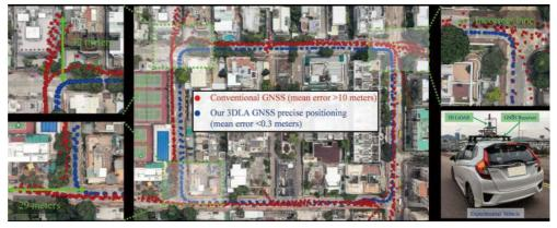
Positioning performance using the 3D LiDAR Aided GNSS Precise Positioning
