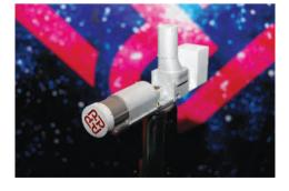
It is compact, lightweight at less than 400 grams, and consumes energy as low as two watts. It could be applied in wide range of environments to support in-situ analysis, which is part of a crucial step in understanding the evolution of the universe. Some of the technologies developed for SOPSYS were applied in the Camera Pointing System.
