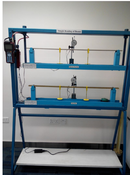
Simple bending of beams
