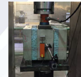
Fig.4 Direct shear test on GFRP shear connector
