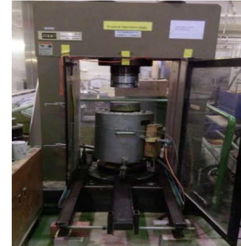
High-Temperature Furnace with MTS 815 Compression Test System
