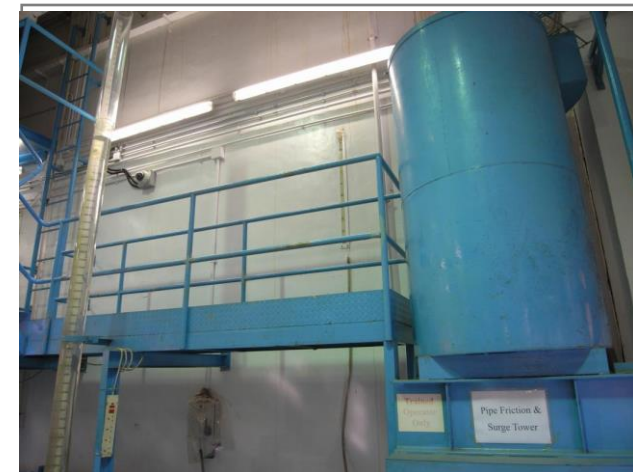
Pipe Friction and Surge Tower
