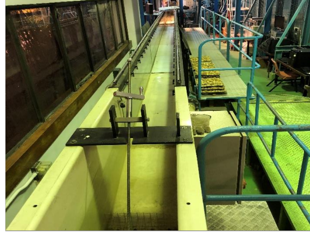
Open Channel (Tilting Flume)
