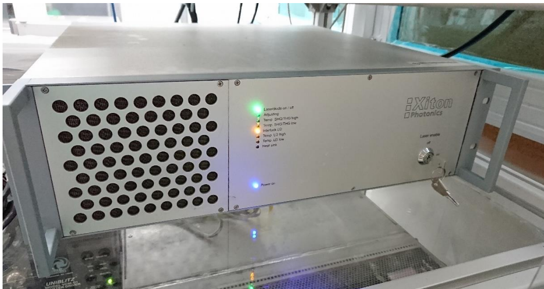
Controller of Xiton Impress 213 Laser
