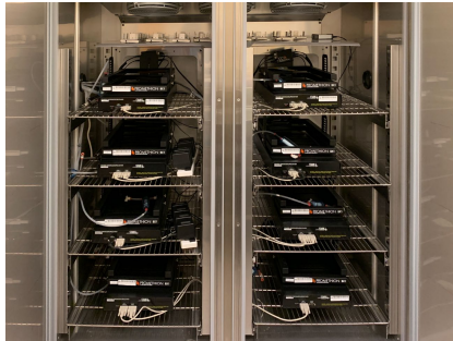
Figure 1. The Sable Promethion metabolic cage system at the ULS comprises 8 cages for individually collecting metabolic and behavioural data of mice over a desired experimental duration.
