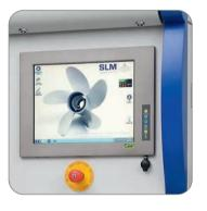
The system is able to process most metals (such as Stainless Steels, Tool Steels, Cobalt Chrome, Aluminum, Inconel and Titanium) through a material saving, closed-loop powder handing unit. Changing the metal powder is quick, easy and designed to lower your production costs.
