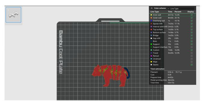
After Slicing, the estimate print time and the material usage will be shown, the printed-out model that including support will also be shown.
