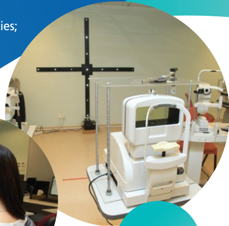
Open-field optical biometer for myopia research
