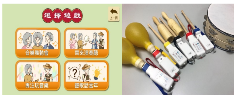
Left photo: The system provides four musical games. Right photo: Specifically designed musical instruments with sensors to track the engagement level and health conditions of the participants.
