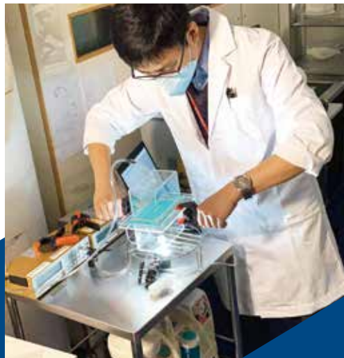
▲ Dr Simon Lam testing the particle filtration efficiency of face masks.
