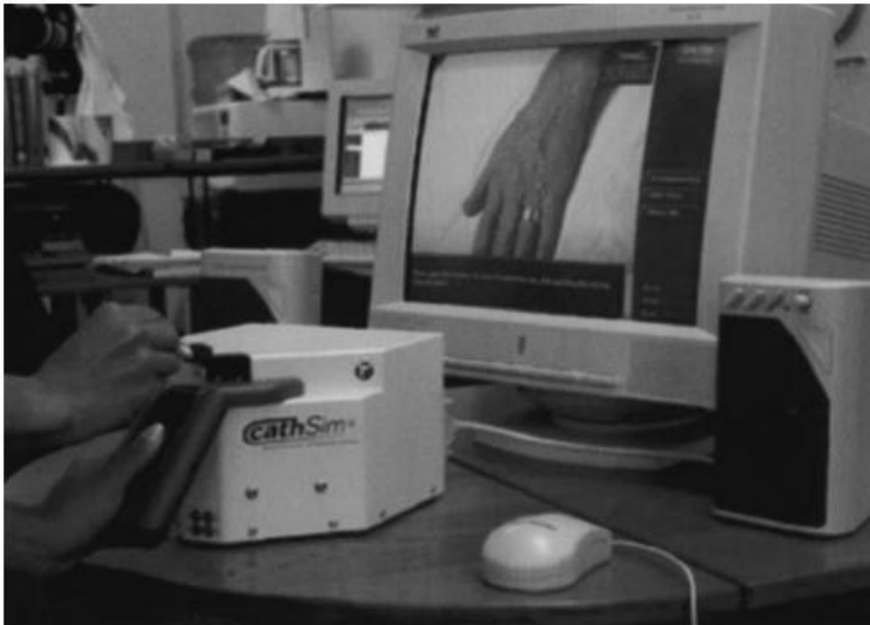
Figure 1. The user interfaces with CathSim via the AccuTouch device. In this figure, the user applies skin traction with her left hand and inserts the IV with her right. In addition to haptic feedback via the AccuTouch device, the user also receives visual feedback from the monitor and audio feedback from the speakers.
