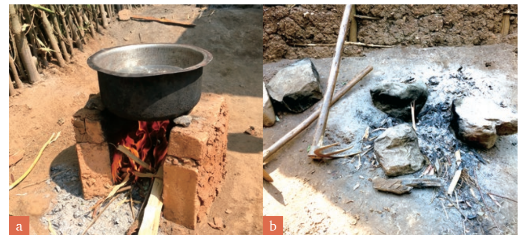
Figure 7-5. (a) A “Rocket” stove built with bricks and mud is cleaner and more efficient, and replaces (b) 3-stone cooking stoves in rural Rwanda, which take a lot of time, consume a lot of vegetation, and generate a lot of smoke and pollution.
