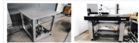
Figure 9. A working bench (Left) and an air anti-vibration bench (Right).
