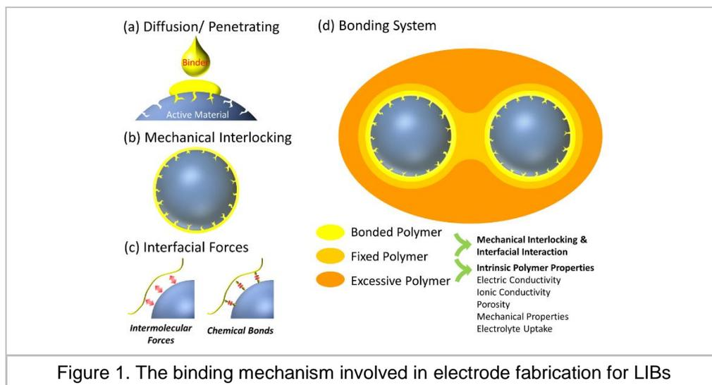
Figure 1. The binding mechanism involved in electrode fabrication for LIBs
