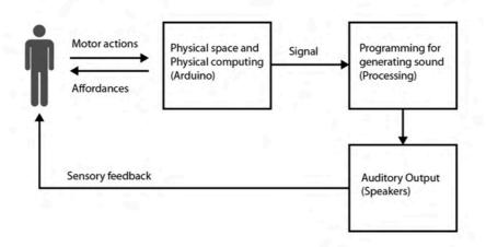
Figure 5.3 Prototype structure of Piano Staircase
