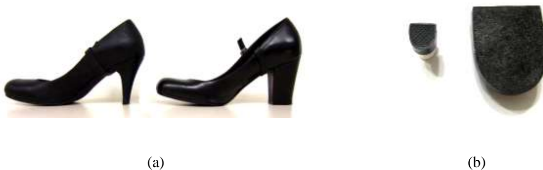
Fig. 1. The experimental shoes with two different HBSs (from left to right: a small size and a large size) (a) Side view of experimental shoes (b) Heel base sizes
