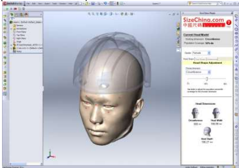
Fig. 8: The design tool running in Solidworks 3D CAD environment
