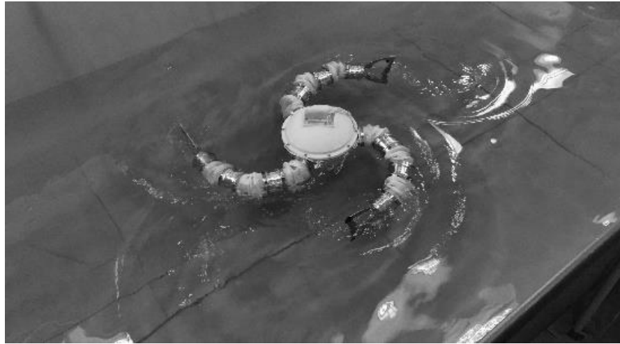
Fig 1. The 2-tail submersible under water robot of capability rotation motion in water without turning radius.
