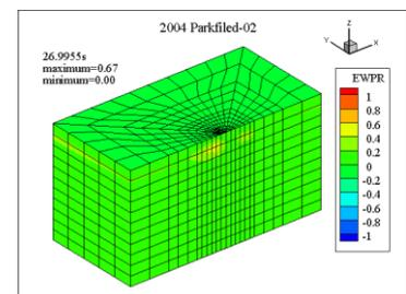
Figure 7 Excess pore pressure ratio of soil domain after the earthquake
