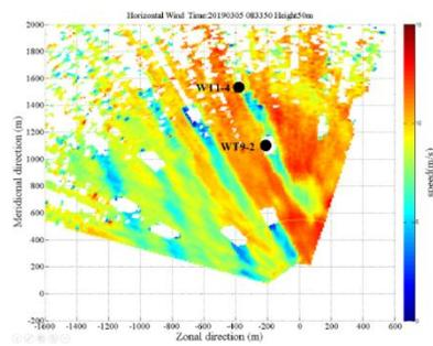
Figure 1 PPI scanning result in the plane at hub height.
