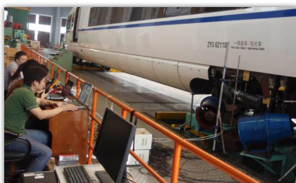
Full-scale vibration control testing using smart dampers for high-speed trains
