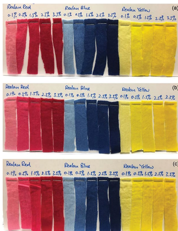
Visual image of dyed wool knitted fabrics in; (a) water, (b) octane, and (c) nonane
