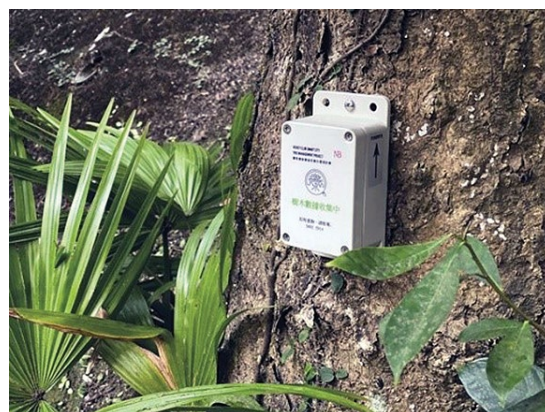
The sensor installed on lower tree trunk for monitoring tilt angles
