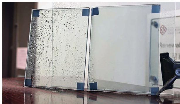
Glass coated with \text{TiO}_2 nanoparticles and ATO
