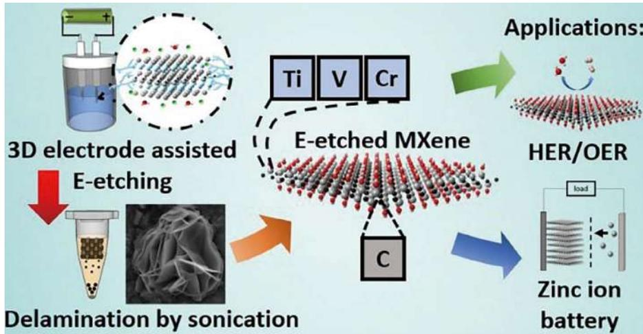
▲ Schematic diagram of fabrication of HF-free MXene
