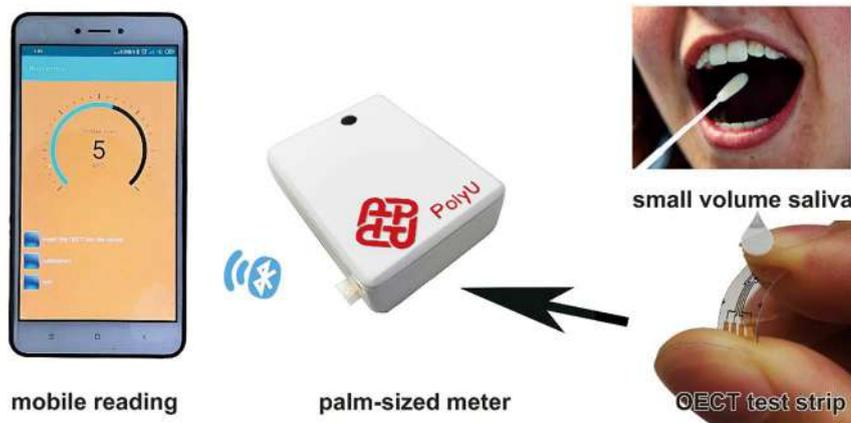
This innovation can realize quick and ultra-sensitive detections of glucose, uric acid or RNA biomarkers for disease diagnostics and virus detection. The most important application is for non-invasive glucose detection in small volume saliva samples, thereby providing a painless and convenient approach for diabetes management.
