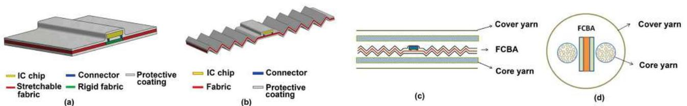
▲ (A) and (B) Two types of schematic FCBA (Fiber-based Circuit Board Architecture) structure; (C) Composite electronic yarn; (D) Cross-section of the composite yarn
