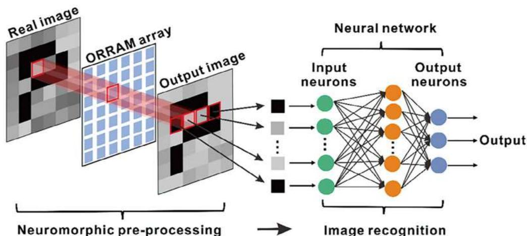
▲ Schematic of an artificial visual system with ORRAM for neuromorphic pre-processing and artificial neural network for image recognition
