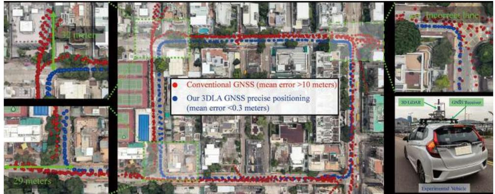
▲ Positioning performance using the 3D LiDAR Aided GNSS Precise Positioning
