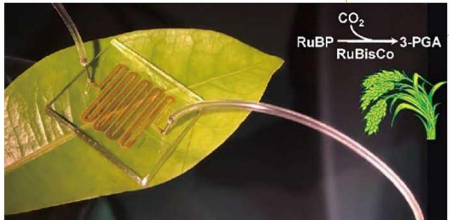
▲ Mimicking photosynthesis, artificial synthesis of carbohydrates are realized from CO<sub>2</sub> using RuBisCO via microfluidic reactors
