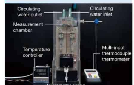
▲ Photo of an apparatus for measuring the thermal conductivity
