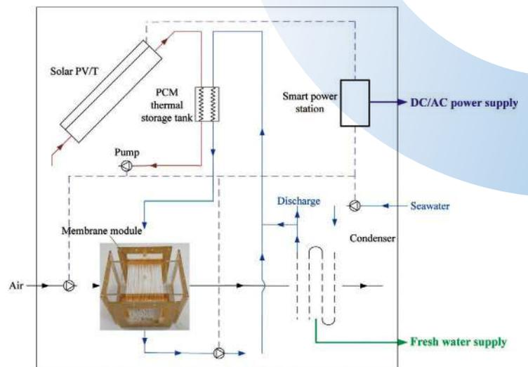
▲ Schematic diagram of the membrane distillation system
