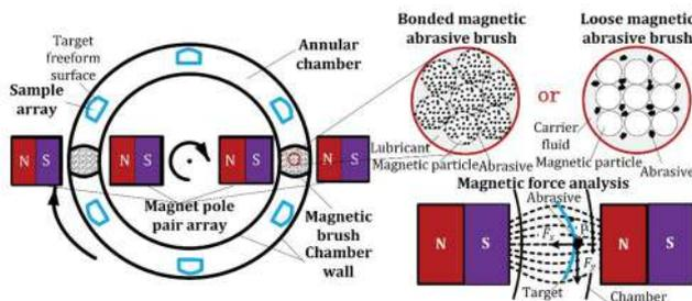
▲ MAMP Schematic Diagram and Experimental Setup
