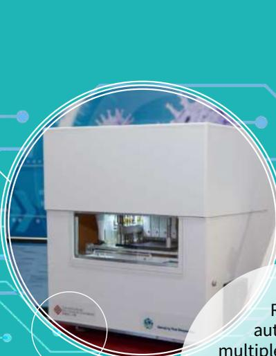
Rapid, automated multiplex diagnostic system for detecting up to 40 infectious respiratory pathogens (including novel coronavirus) in a single test
