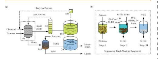
The technology aims to fractionate high-value lignin from wastes derived lignocelluloses. The overall biomass conversion is conducted by mixing the biomass with 1,4-butandiol (BDO) in reactor operated under a sequencing batch reactor mode for pretreatment, cellulose regeneration, and enzymatic hydrolysis. The regenerated substrate will be subjected to hydrolysis and the solvent in the spent liquor will be recycled.
