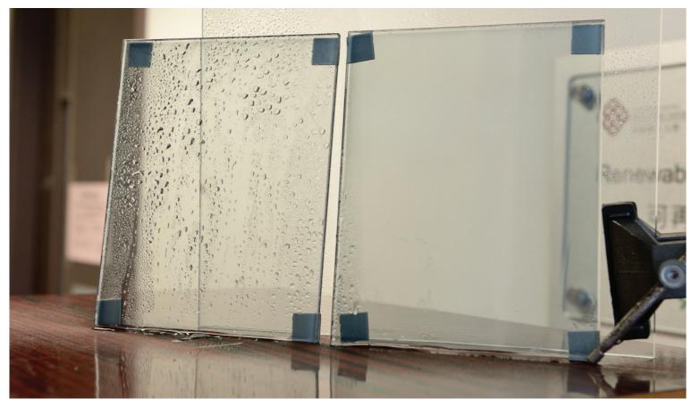
A novel long-term glass multi-functional layer is developed by uniform coating nanoscale  $TiO_2$  and Antimony doped tin oxide (ATO) mixture particles as the main material on various glasses. The  $TiO_2$  nano-particles are synthesized by low-cost hydrothermal method while the ATO by high-temperature calcination technique.
