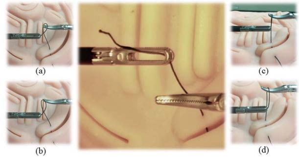
Fig. 3. (a) and (b) Suture's slack and slippage while winding. (c) and (d) Collisions of the gripper with the suture.
