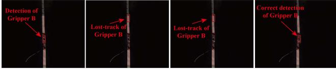
Fig. 15. Lost tracking of grippers in the suture looping process.
