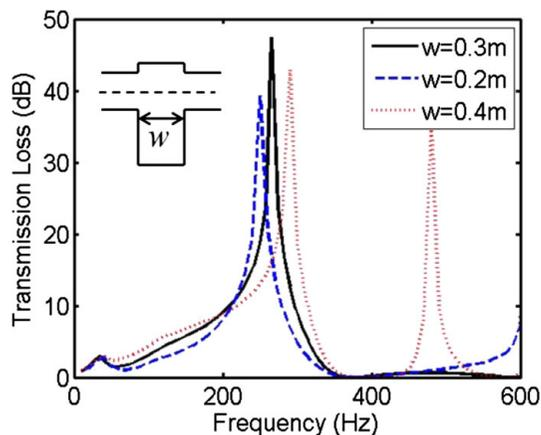
Fig. 4—Effect of varying width,  $w$ , of an empty sub-chamber.
