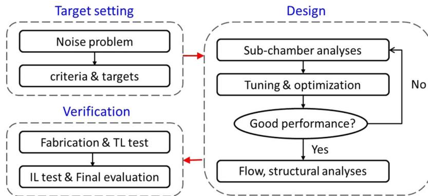
Fig. 13—Flowchart of the cascade muffler design.
