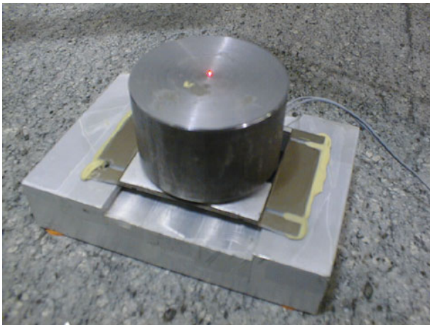
Figure 1. The THUNDER with 500 g load on the apex and with both ends fixed with silicone gels.
