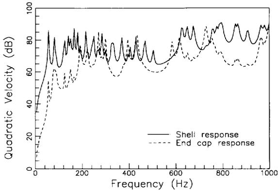
Fig. 3. Quadratic velocity of the vessel containing water.
