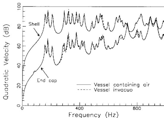
**Fig. 2.** Quadratic velocity of the vessel in air and *in vacuo*.
