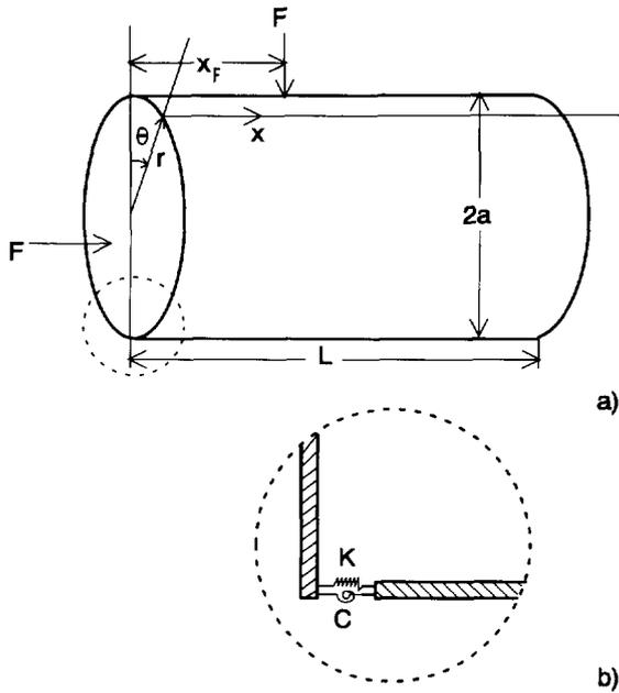
Fig. 1. Investigated structure and spring set-up.
