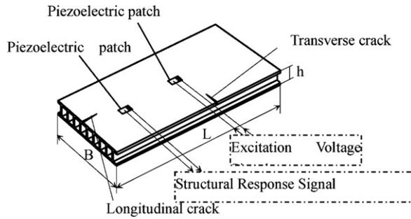
Fig. 2. A honeycomb sandwich plate with crack damage [44].
