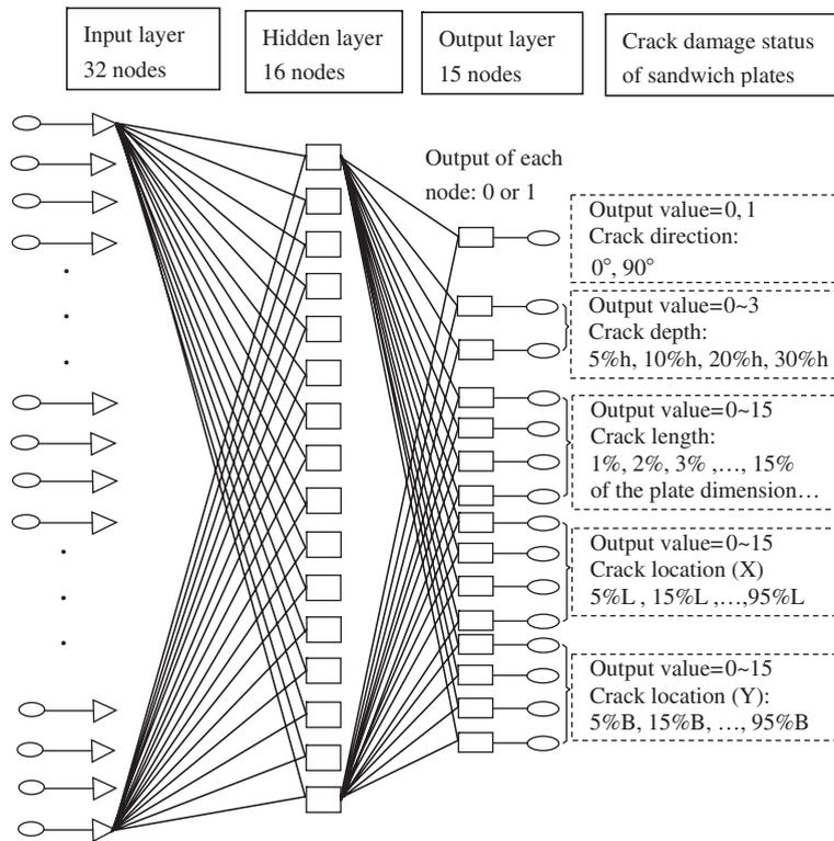
Fig. 3. BP neural network for identification of multiple crack parameters [44].
