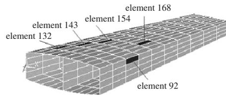
Fig. 4. A composite airfoil case model and the given damage status.
