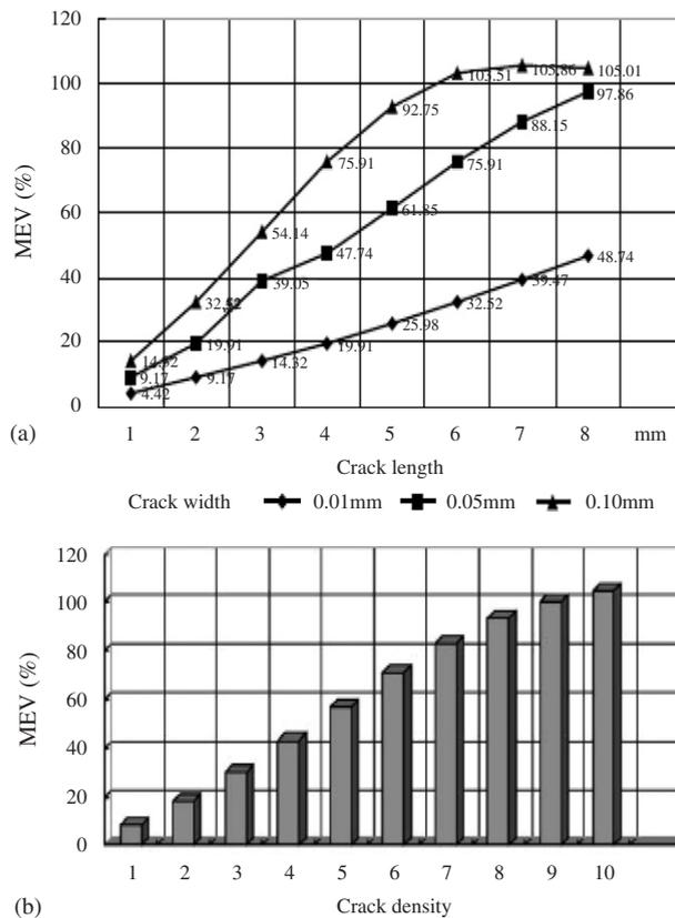
Fig. 1. Damage severity vs. the constructed damage feature index [36].
