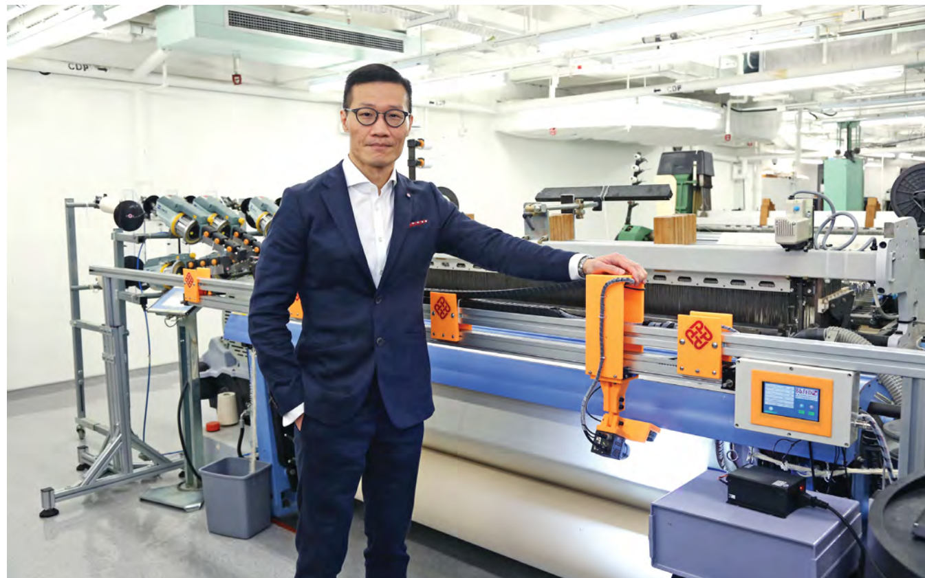
The WiseEye system, developed by Prof. Calvin Wong, is equipped with a camera that can move back and forth on a weaving machine to capture images of the whole width of woven fabric.
