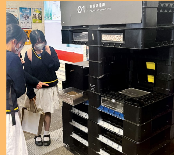
The JAP JAP system features various stackable, upcycled plastic pallets that can be configured into different sizes to fit different needs and environments.
