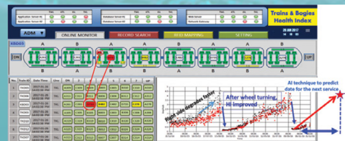
Computer user interface for the track-based train condition monitoring system
