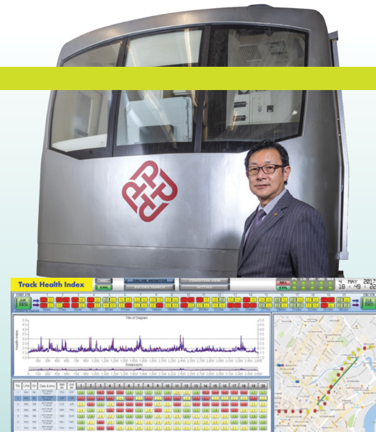
Computer user interface for the train-based track condition monitoring system
