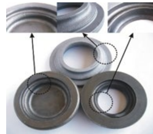
Figure 3: Folding defects in macro-scaled flanged parts
