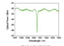
聚合物光纖光柵透射譜 Transmission spectrum of polymer fiber Bragg grating
