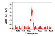
聚合物光纖光柵反射譜 Reflection spectrum of polymer fiber Bragg grating
