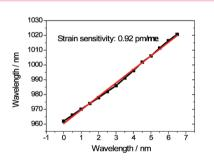
聚合物光纖光柵應變輸出 Strain response of polymer fiber Bragg grating
