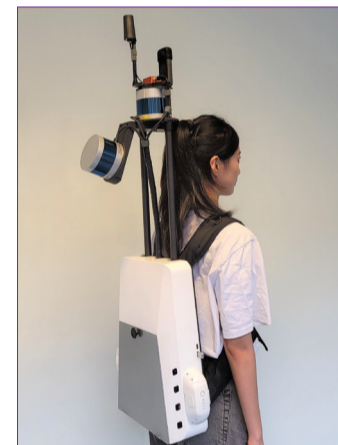
輕量級三維空間數據採集系統 (移動測圖背包) Lightweight 3D spatial data acquisition system (mobile mapping backpack)
