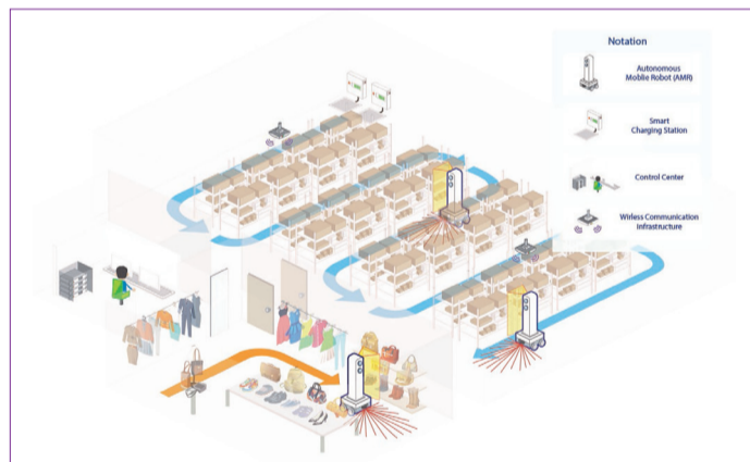
基於AIoT技術的庫存審計和自主移動機器人監控系統概念圖 Conceptual diagram of the AIoT-based Inventory Auditing and Surveillance Autonomous Mobile Robot System
