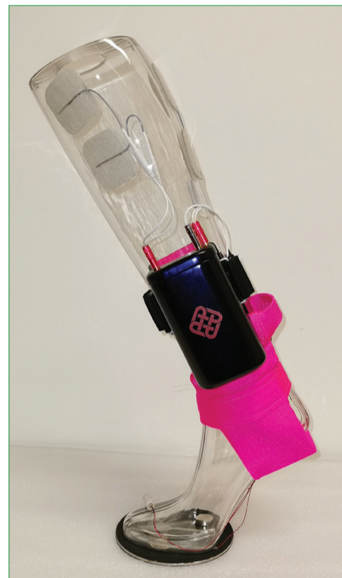
智雲行健步儀 The mobile ankle-foot exoneuromusculoskeleton
