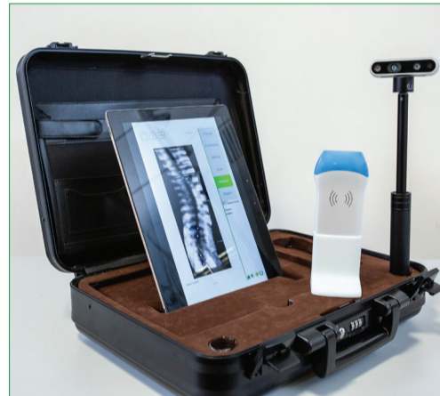
便攜式的三維超聲成像系統 Portable 3D Ultrasound Imaging System
