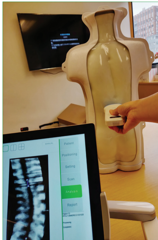
便攜式超聲探頭 Palm-sized ultrasound probe
