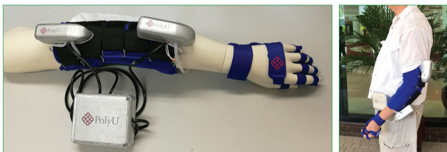
移動式外神經肌骨系統具高度彈性布料，患者可舒適地穿戴著進行訓練 Mobile Exo-neuro-musculo-skeleton has a highly flexible fabric interface and can be worn comfortably
