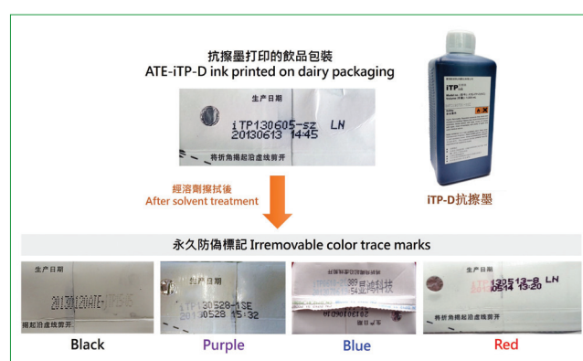
雙層雙色納米抗擦墨經過溶劑擦拭後的防偽效果 Anti-counterfeit effect of ATE-ITP-D inks after solvent treatment
