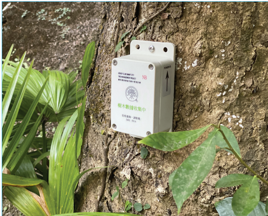
安裝於樹幹較低位置的傳感器監測樹木的傾斜角度 The sensor installed on lower tree trunk for monitoring tilt angles
