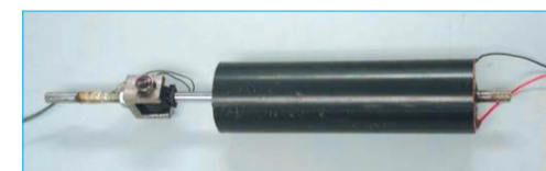
系統應用於斜拉索的振動控制 Application of the smart system to Vibration Control of the Stay Cables in a Cable-Stayed Bridge
