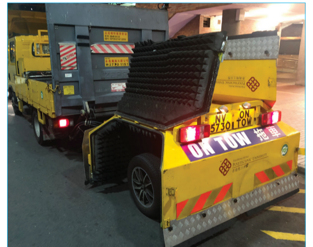
可持續低噪音路面已接受近距離路面噪音測量車測試，證明其路面噪音比傳統瀝青路面低三分貝 Sustainable low-noise pavements were tested with a close-proximity (CPX) trailer and proven to generate tyre-road noise which is 3dB less than that of conventional asphalt pavements
