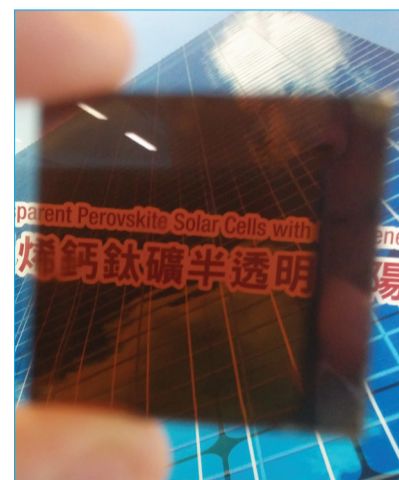
石墨烯鈣鈦礦半透明太陽能電池 Semitransparent perovskite solar cell with graphene top electrodes
